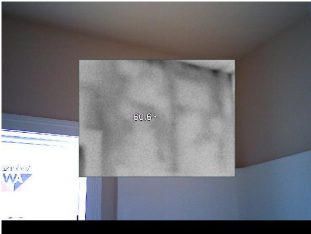
This wall's dense pack looks a little off – its not as consistent as all the others. Minor – but noteworthy.
